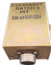
Ks2 Steering Lamp Control Box
